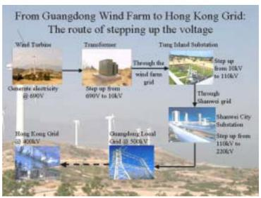
Figure 1. From GuangdongWind Farm to Hong Kong Grid: the route of stepping up the voltage<sup>2</sup>
